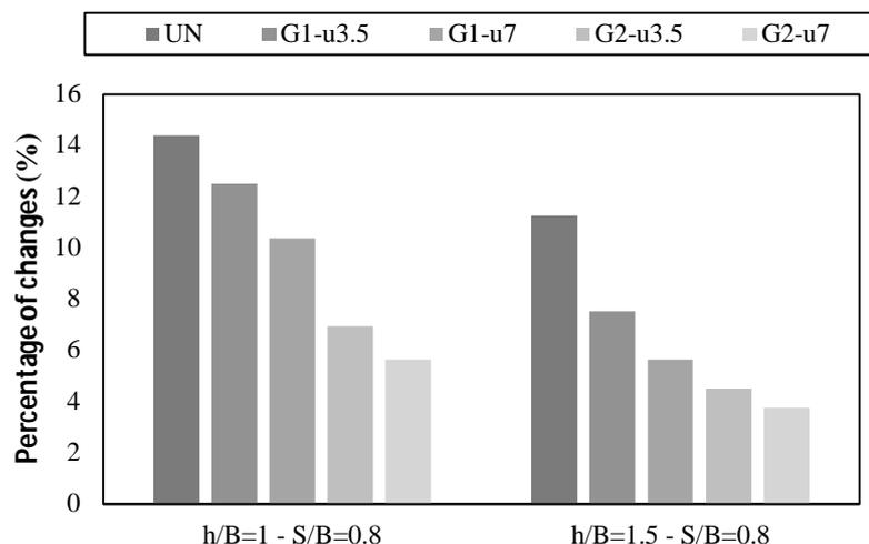
Fig. 3. Graph of the percentage variations in the horizontal spacing between voids in dense soil with reinforcement under different conditions
