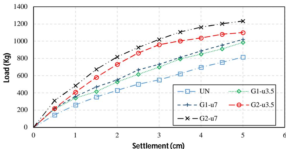
Fig. 1. The load-settlement curve of loose soil with twin voids with ratios of  $h/B=1$  and  $S/B=0.6$
