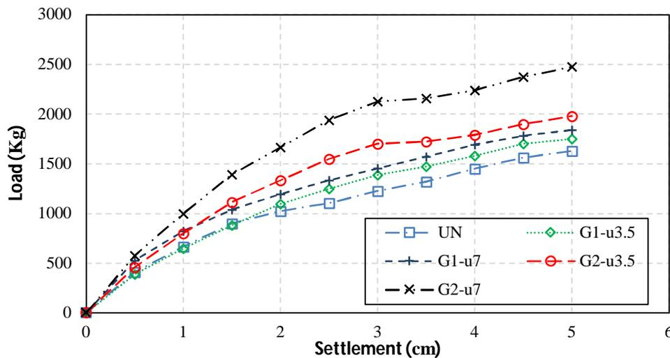
Fig. 2. The load-settlement curve of dense soil with twin voids with ratios of  $h/B = 1.5$  and  $S/B = 0.8$
