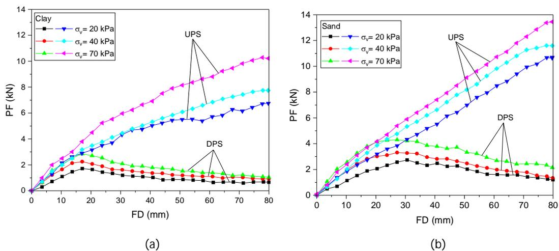
Fig. 2. Variation of pullout force of DPS and UPS in uniform (a) clay and (b) sand with respect to frontal displacement
