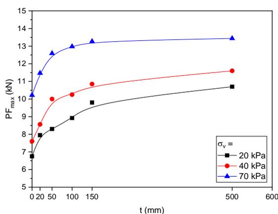
Fig. 3. Variation of pullout strength with respect to the thickness of sand layer in sandwich method
