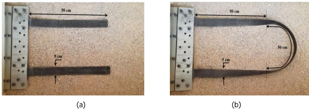
Fig. 1. Strap configuration (a) DPS (b) UPS
