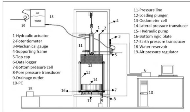
Fig. 1. Schematic representation of the large oedometer system
