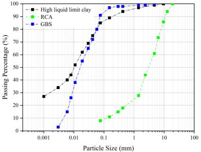
Fig. 1. Particle size distribution curves of the tested clay, RCA and GBS
