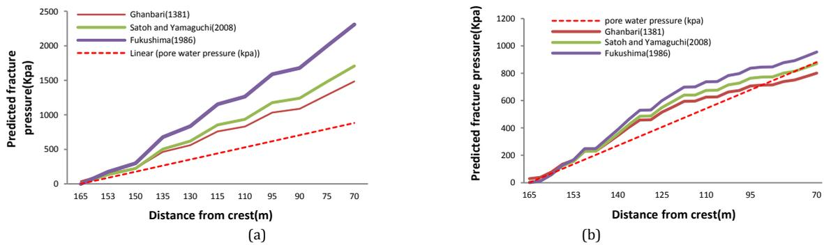
**Fig. 1.** (a) Comparison of hydraulic fracture pressure for CH soil in the stage of steady state in section A-A, (b) Comparison of hydraulic fracture pressure for CL soil in the stage of steady state in section A-A
