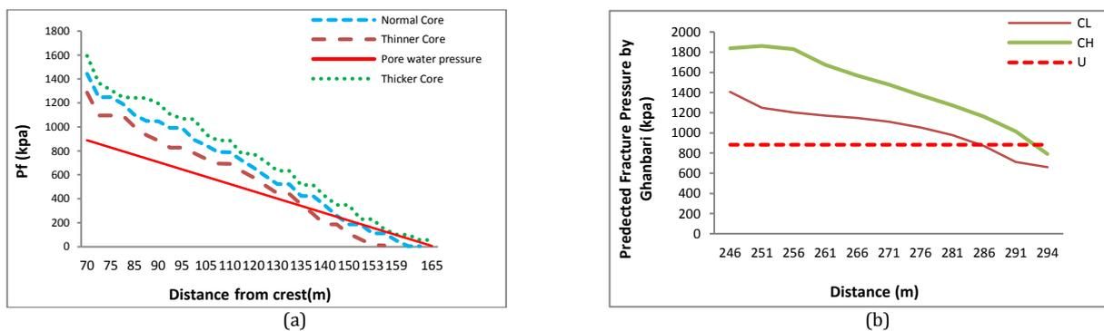
**Fig. 2.** (a) Comparison of fracturing pressure (kpa) in the dam considering thinner and thicker core based on simple tensile criterion (CH), (b) Investigating the possibility of hydraulic failure at the bottom of the core based on the Ghanbari shear criterion (2009)
