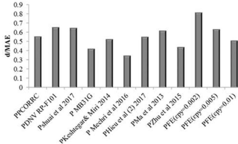
**Fig. 1.** Comparison diagram of finite element models based on Ramberg-Osgood relationship with experimental models using d/MAE criterion
