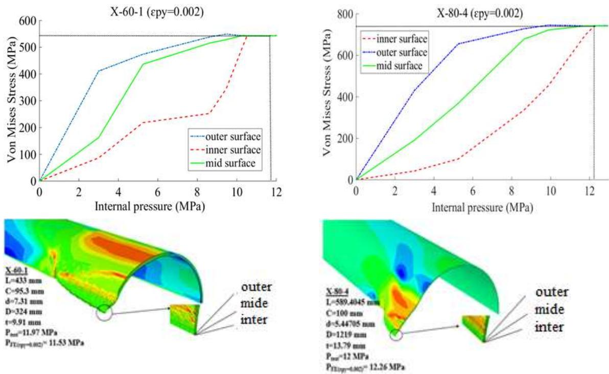
Fig. 1. The burst pressure of corroded pipe according FEM based on the Ramberg-Osgood relationship
