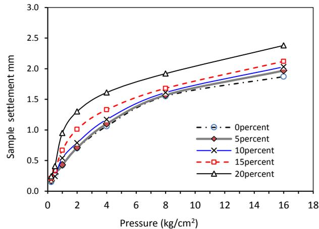
**Fig. 6.** The settlement curves of the soil samples with different amounts of oil at different pressures during consolidation tests
