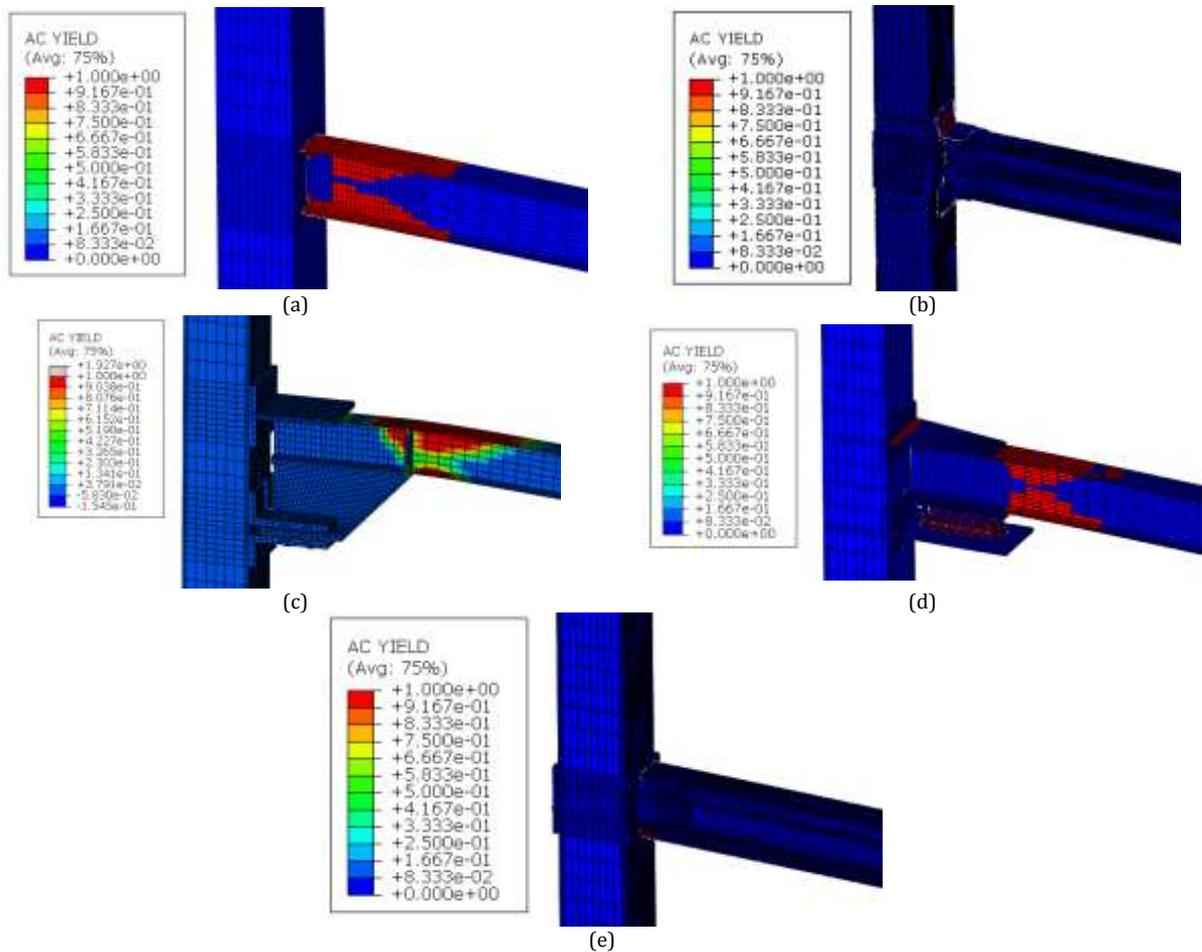
Fig. 1. Yielding status of the models at the rotation of 0.06 Rad: a) WMC, b) PTSC, c) FDC, d) MYDC, e) SCPCFD
