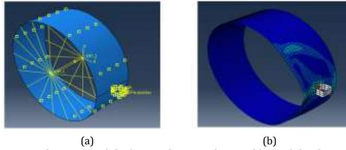
Fig. 1. Finite element model: a) Boundary conditions, b) Final displacement
