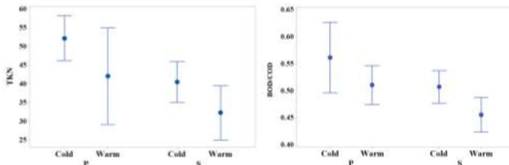
**Fig. 1.** TKN concentration (left) and BOD/COD ratio (right) in effluent of facultative ponds in series (S) and parallel (P) formation in cold and warm seasons
