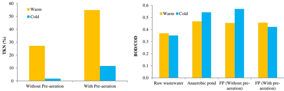
**Fig. 2.** TKN removal (left) and BOD/COD ratio (right) of Delijan WWTP with parallel facultative ponds (FP) with and without pre-aeration in cold and warm seasons
