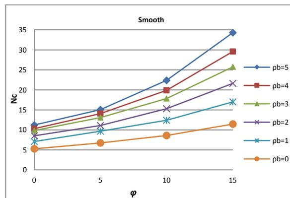
Fig. 2. Bearing capacity factor  $N_c$  against different values of  $\rho$
