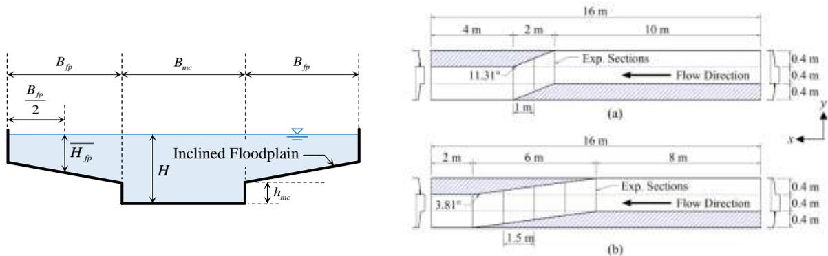
**Fig. 1.** Plan view and cross-section view of skewed compound channel with inclined floodplain
