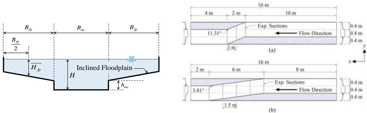
**Fig. 1.** Plan view and cross-section view of skewed compound channel with inclined floodplain
