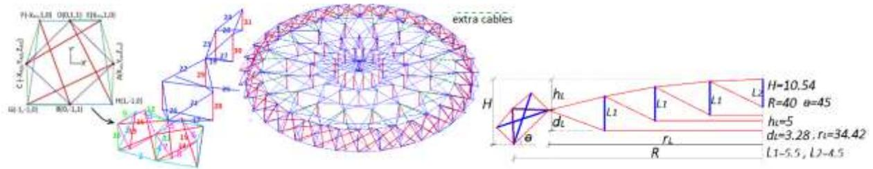
**Fig. 1.** The semi-regular tensegrity module and the hybrid structure with geometric characteristics and elements grouping
