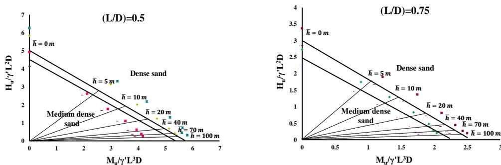
Fig. 1. Normalized ultimate horizontal load-overturning moment diagrams (Embedment ratio=0.5; up left, Embedment ratio=0.75; up right, Embedment ratio=1; down).
