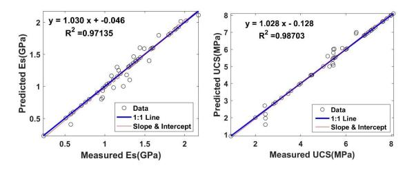
Fig. 2. Relationship between measured and estimated parameters by SVR method (for all data)
