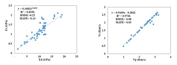
Fig. 1. Relationship between static elastic modulus and shear wave velocity with dynamic properties
