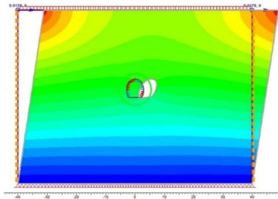
Fig. 1. Distribution of rock mass displacements and yielded lining elements
