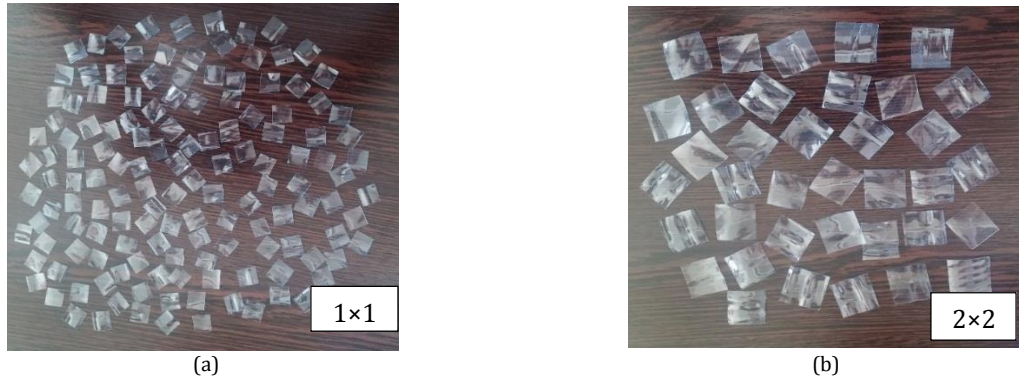
Fig. 1. Image of PET plastic waste strips: a) 1×1cm, b) 2×2cm
