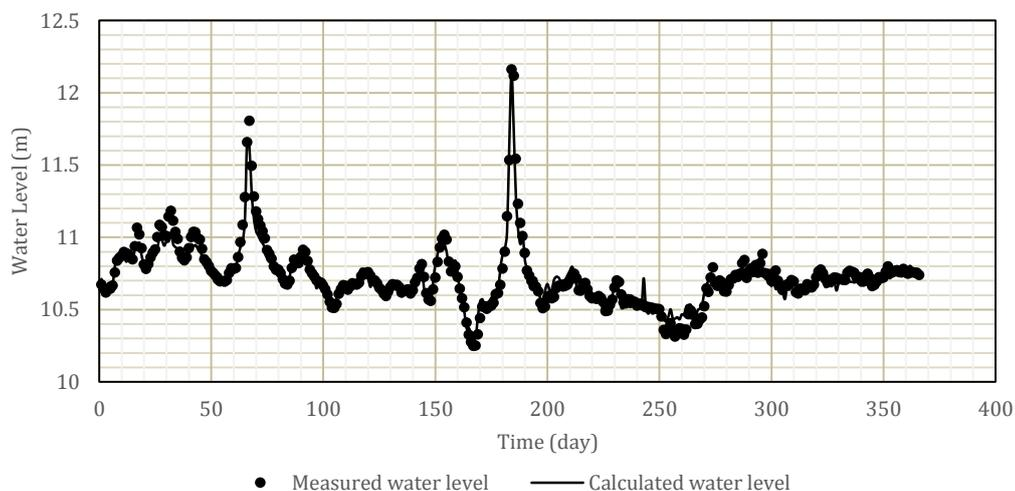
Fig. 3. Comparison of modeling and measured water level in Ahvaz station
