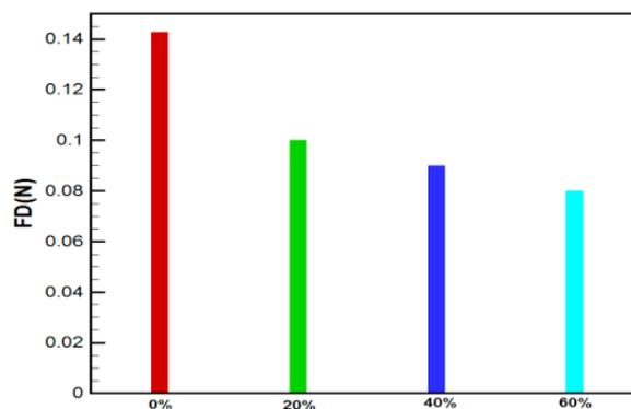
Fig. 1. Bar graph of the drag force applied to the gabion groines with different porosity percentage
