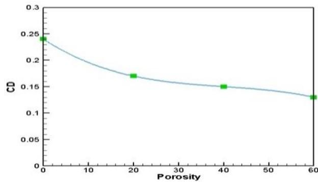
Fig. 3. Variation of drag coefficient with porosity percentage for side obstacles using power law scheme
