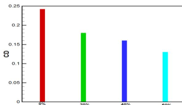
Fig. 2. The bar graph of the drag coefficient of gabion groines with different porosity percentage
