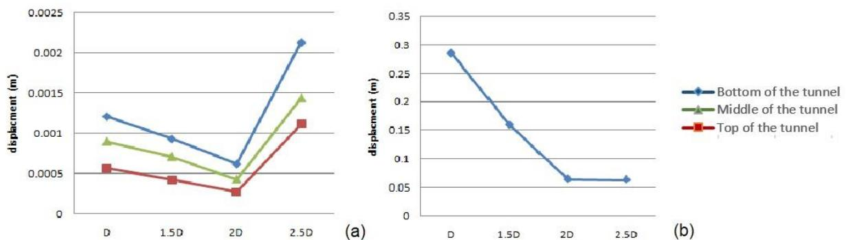
**Fig 1.** a) Effect of the distance between the piles and the tunnel to move the tunnel in the longitudinal direction, b) Effect of the distance between pile group and the tunnel on displacement of pile group in the direction of earthquake
