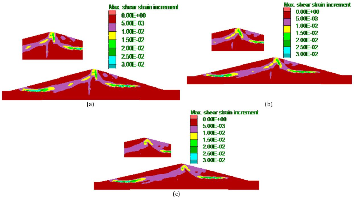
Fig. 3. Shear strain zone whit: a) angle of 90 degrees, b) angle of 100 degrees, c) angle of 110 degrees
