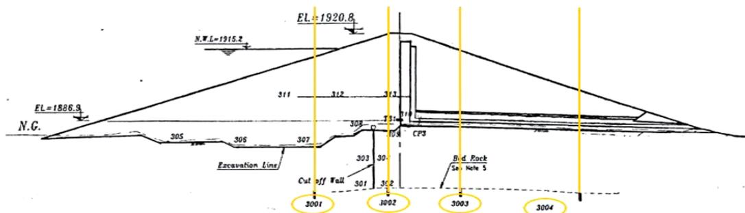
Fig. 2. The cross-section of the Malayer dam
