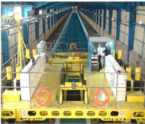
Fig. 1. Wave flume and manned chariot of NIMALA marine laboratory
