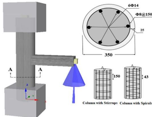
Fig. 2. Finite element model of the equivalent column
