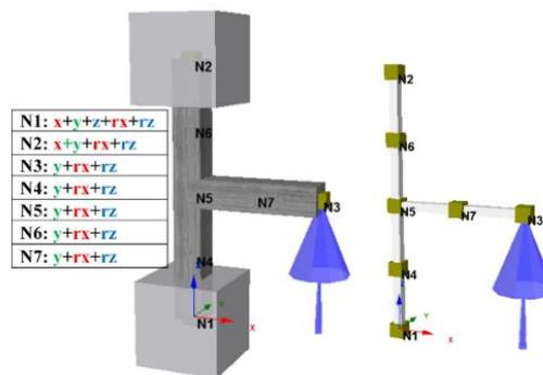
Fig. 1. Finite element model of the specimen
