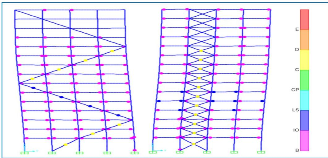
Fig. 2. Example of the condition of the plastic hinges at the target displacement for the rehabilitated structures
