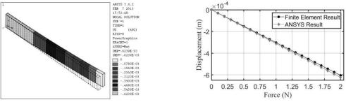
Fig. 4. Comparison of proposed finite element model and ANSYS: load-displacement
