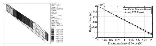
Fig. 6. Comparison of proposed finite element model and ANSYS: electromechanical-displacement
