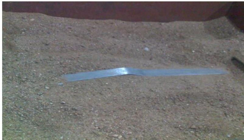
Fig. 1. Plastic deformation after pull out test
