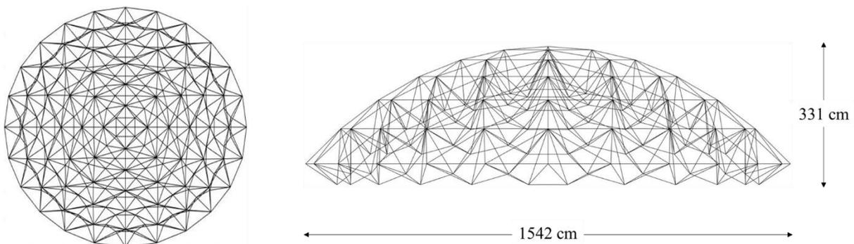
Fig. 1. Dimensional characteristics of the investigated structure
