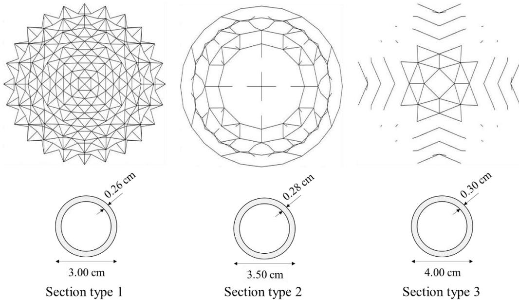
Fig. 2. Section profiles used for structural elements
