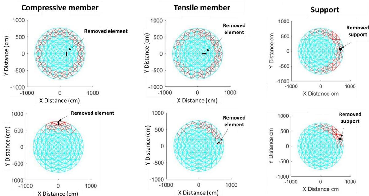
Fig. 6. Pattern of progressive collapse for elimination of compressive members, tensile members and supports
