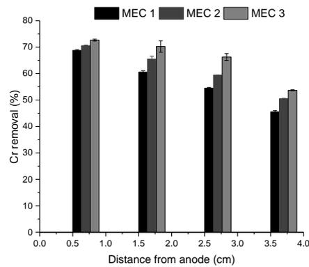
**Fig. 4.** Chromium removal within the sediment sample
