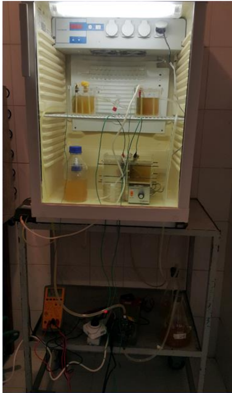
Fig. 1. Set up of dual chamber microbial fuel cell
