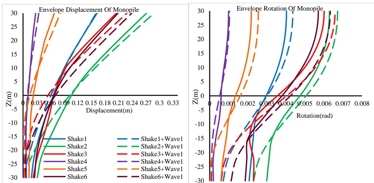
Fig. 2. Effect of the wave on the seismic displacement & rotation of monopile
