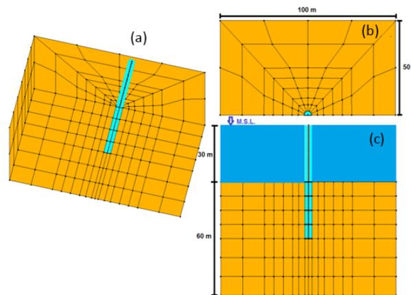
**Fig. 1.** FE mesh of the developed numerical model: schematic illustration in medium dense sand subjected to the wave and earthquake loading
