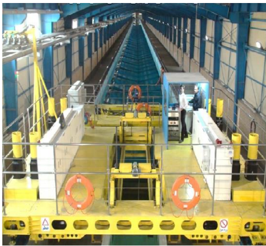
Fig. 1. Wave flume and manned chariot of NIMALA marine laboratory
