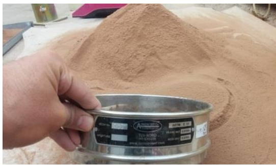
Fig. 2. Image of fin-grained soil in present study: a) passed from sieve No. 100, b) grain size distribution
