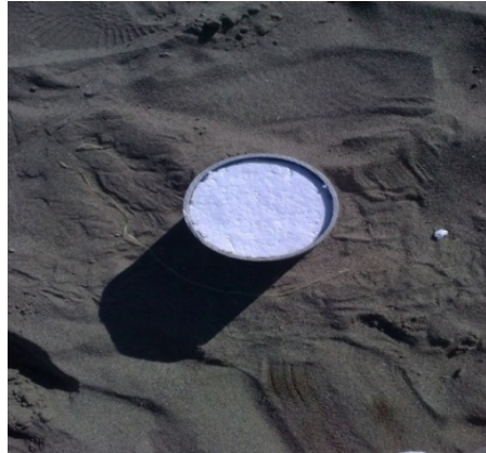
Fig. 1. Placing of yunolit in the inside of the pvc pipe
