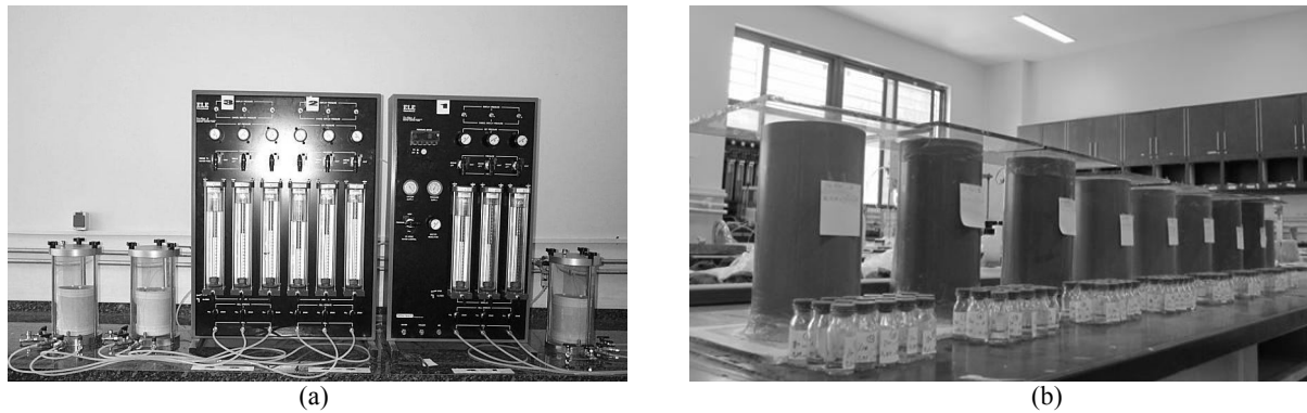
Fig. 1. Hydraulic conductivity and diffusion tests: (a) Triaxial hydraulic conductivity apparatus with three BES samples in the test cells, (b) Diffusion cells with NaCl samples taken during the diffusion tests.
