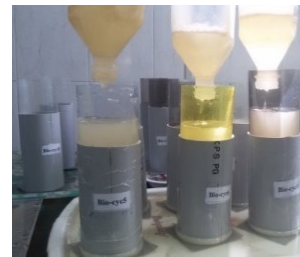
Fig. 3. Injection of cementation solution into soil samples by gravity method
