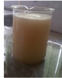
Fig. 2. cementation solution of 0.5 M urea and 0.5 M calcium chloride
