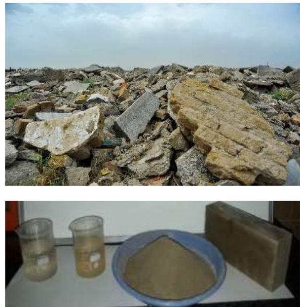
**Fig. 1.** Demolishing waste containing CBW (Top), and CBW powder, alkaline solutions and CBW-based geopolymeric brick (Bot)
