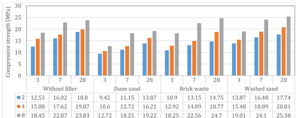
**Fig. 8.** Compressive strength of geopolymer bricks with WG/NaOH=2
