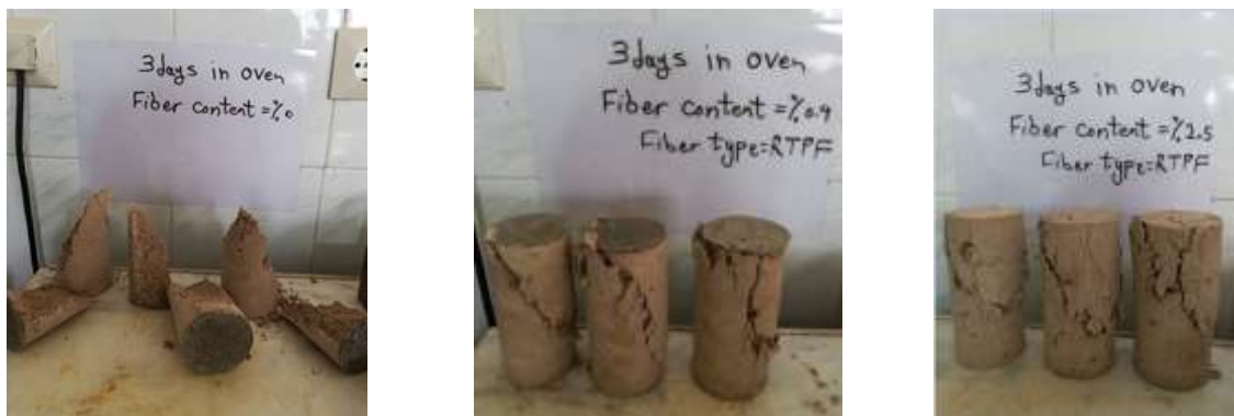
Fig. 1. A view of typical specimens after failure (cured at 60°C)
