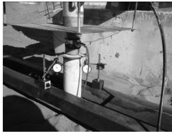
Fig. 2. Instruments for measuring load and displacement
