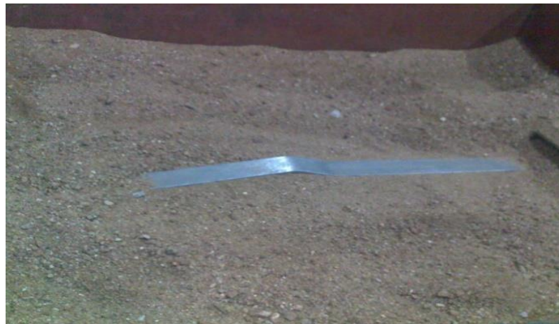
Fig. 1. Plastic deformation after pull out test
