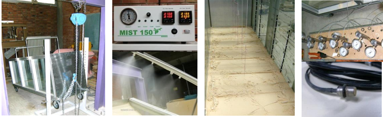
Fig. 1. Test setup: a) Flume box and lifting system, b) Rainfall controlling unit, c) Misting (rainfall) sprinklers, d) instrumentation placed in soil sample, e) gauges of tensiometers, f) pore pressure transducers
