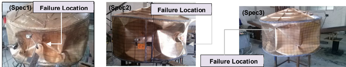
Fig. 3. (a) Full buckling of Spec1 and instability threshold, (b) Failure of the Spec 1.
