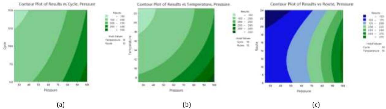
**Fig. 1.** (a) Changes in the maximum deviatoric strength according to the confining pressure and the number of freeze-thaw cycles, (b) Changes in deviatoric strength in terms of confining pressure and temperature of freeze-thaw cycles, (c) Maximum changes in deviatoric strength according to confining pressure and temperature of freeze-thaw cycles
