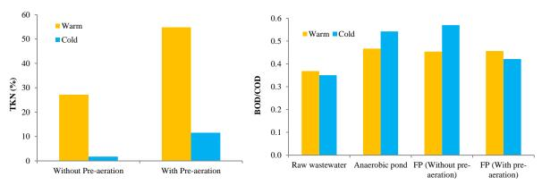
Fig. 2. TKN removal (left) and BOD/COD ratio (right) of Delijan WWTP with parallel facultative ponds (FP) with and without pre-aeration in cold and warm seasons
