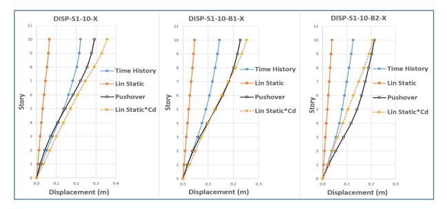
Fig.3. Comparison of the floor displacements predicted using linear and nonlinear analyses for the S1-10 structure in X direction
