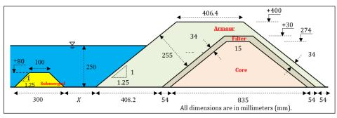
Fig. 1. Transversal section of the wave flume and the position of the breakwater and the obstacle
