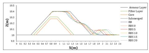
Fig. 2. Reshaped Rubble mound breakwater profiles in all test modes
