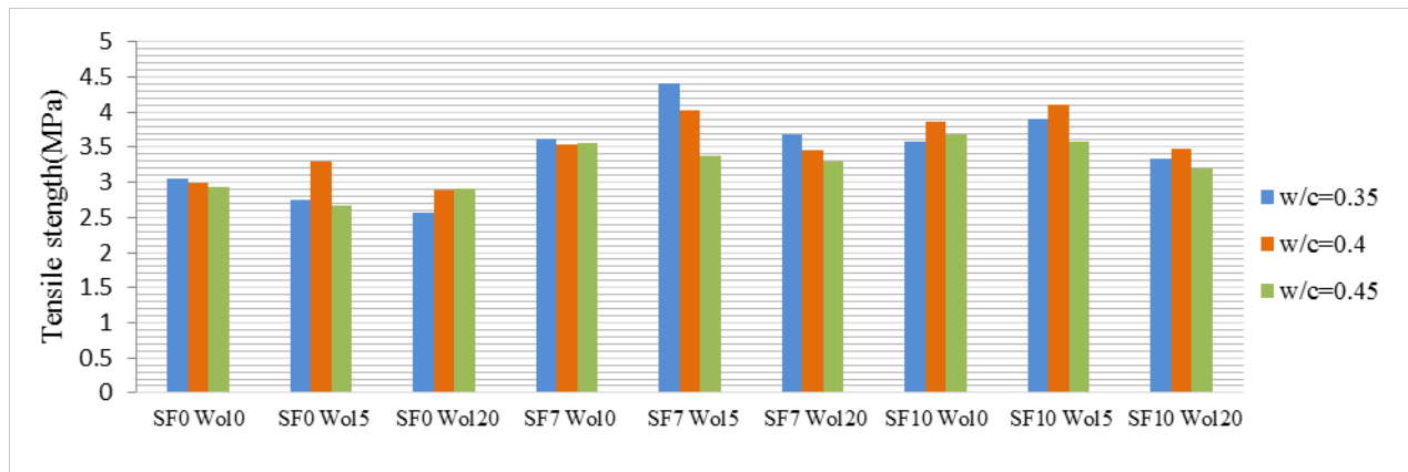
Fig. 1. Tensile strength at the age of 28 days
